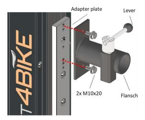
Screw the enclosed bolt into the clamp. Fasten the bolt hand - tight.
