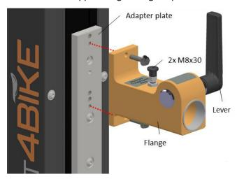
Insert the clamp into the flange:
