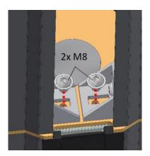
Screw the crossbar tight with the two M8 screws supplied.
